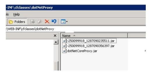
Of course, one of the Jar files that ColdFusion creates is the actual assembly interface which "mirrors" the methods and properties of the .NET interface. It's the one with the cryptic name that looks like "-23480983\_3023903.jar". The other file however is special. It's the one that is always named dotNetCoreProxy.jar. It is compiled only once (unless you delete it) on the first time you instantiate a .NET assembly. It provides (presumably) the interface to the proxy listener.
